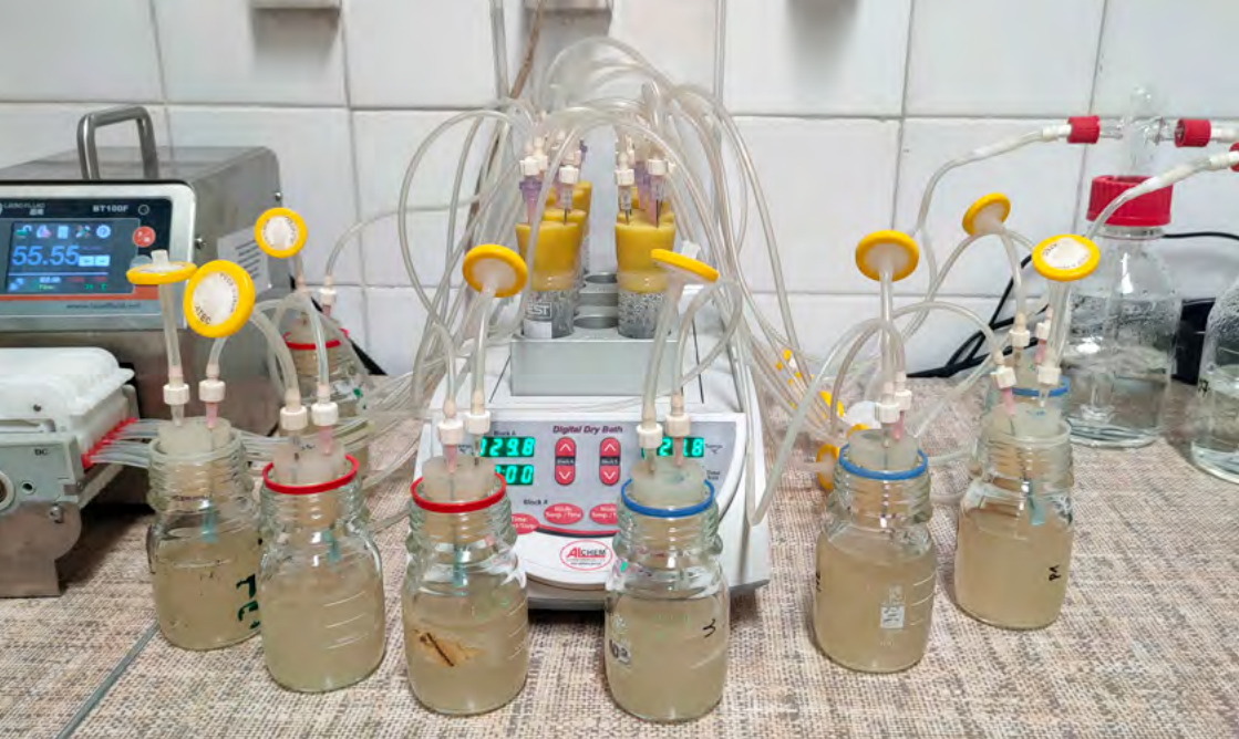
| Multiplexed self-made chemostat (with controlled temperature, medium and air flow).
