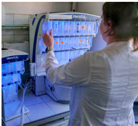
Automatic peptide synthesizer at work (with Ms. Dobromiła Sudzik, Ph.D. student)
